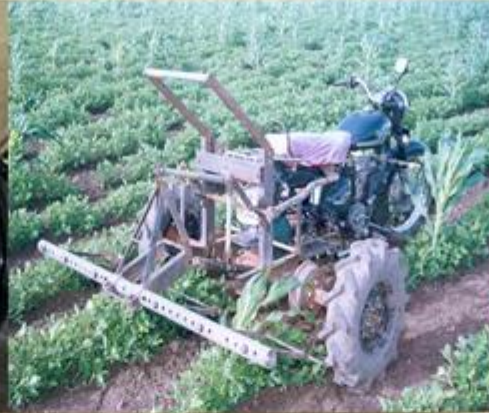
Motor-cycle based ploughing attachment 'Bullet-Santi' Mr. Mansukhbhai Jagani, Gujarat
