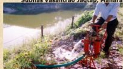
Bicycle based portable Pump, Mr. Nasiruddin Gayen, WB
